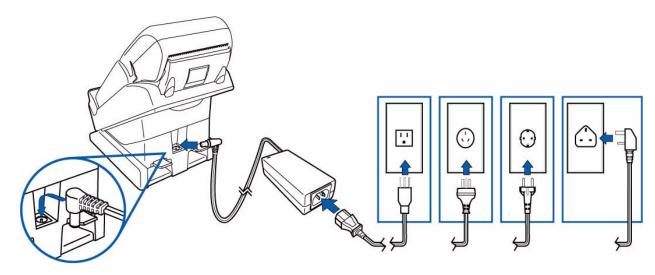
Figure 22 Connecting the Base Station to a Power Source
